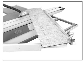
Figure 64. Example of miter cutting operation.
